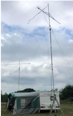
2m & 70cm beams at M5MK/P VHF NFD station
